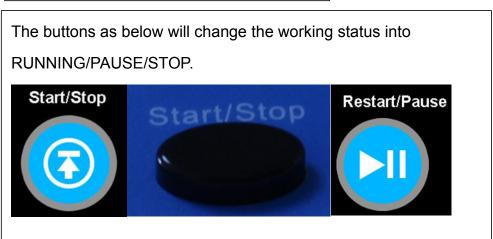
D.Press Start/Stop Button(either Main screen or User facing screen button) to activate the light.
